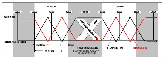
Figure 3: Conceptual time table with two trainsets providing 1 800 seats per direction per day
