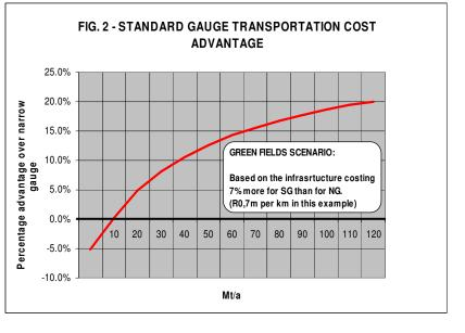
From 10 Mt/a upwards the standard gauge advantage in unit transportation cost increase to about 10% at 30 to 40 Mt/a and to about 20% for traffic volumes exceeding 100 Mt/a.
