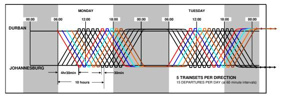
Figure 4: Conceptual time table with ten trainsets providing 9 000 seats per direction per day
