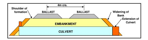
Another alternative would be to do the extension on one side only. The centre lines of the tracks would then have to be moved. Such extensions could then be done with heavy earthmoving equipment to a minimum width of approximately 2.5 meters. Fairly substantial benching could then be done into the existing embankments without endangering the tracks on the embankments. This method would however also require moving of the electrification masts and other structures.
