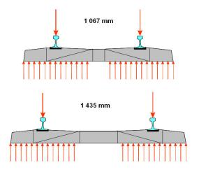
machines. The centre portion of the sleeper provides minimal to zero vertical support as per the adjacent sketch, although it does provide higher resistance to cross-level disturbance.
