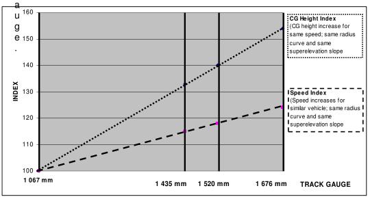
It would appear unlikely that double stacking of loaded containers on narrow gauge wagons will become feasible<sup>6</sup>.
