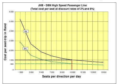
The figure above projects a cost per seat-trip of R1 000 at a volume of about 11 000 per direction per day (for a discount rate of 8% p.a.) With sufficient freight trains to contribute to the revenue this rate could be stable at R1 000 per seat-trip for all volumes down to 1 800 per direction per day.
