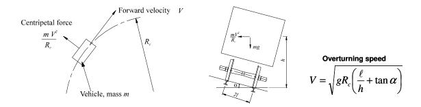
The formula provides the critical overturning speed for a rigid vehicle. The actual situation is complicated by the fact that vehicles are not rigid. The actual overturning speed for a sprung vehicle is generally about 20% below that provided by the above simplified formula.
