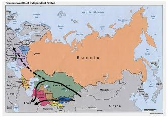
The BG Trans-Siberian-Railway is currently a growing landbridge moving traffic from Japan and China to Europe. Such traffic still has to cope with breaks of gauge upon entering into the European SG network, and depending on origin, between China and Russia.
