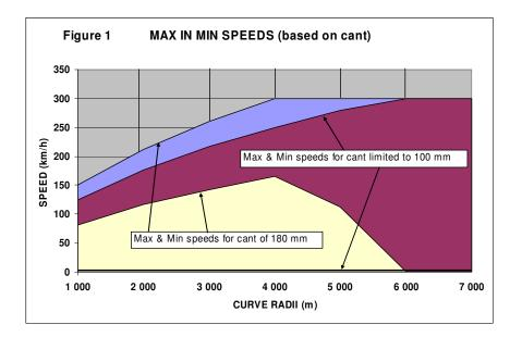
Figure 1 indicates the maximum and minimum speeds around curves for different cant conditions. The UIC task team on high speed lines recommended a maximum cant of 180
