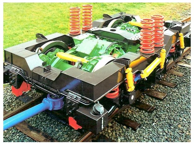
Figure 1: A motored bogie<sup>5</sup>
